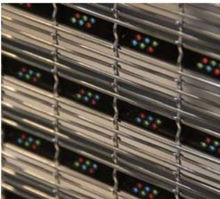
**FLEXIBILITY** Multiple customization options including LED profile length, number of pixels (from 8 to 72 LED pixels per profile piece), and the configuration and location of each LED profile, can be custom selected. The linear LED configurations are easily attached to the steel mesh with a patented clip system, allowing easy installation and maintenance of the LED tubes.
